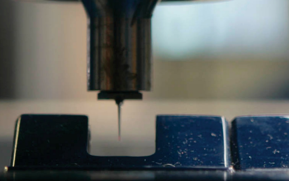
'window waste' with ultra sonic cutting
